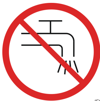
Figure 104 – Warning symbol: Machine not suitable for connection to the potable water mains
