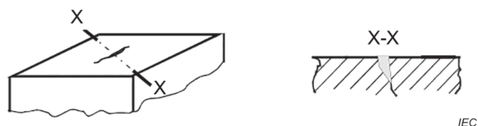
Figure 11 – Single-surface broad crack
