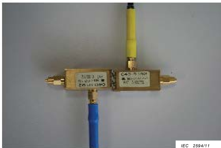
Figure 12 – Configuration for balun CM insertion loss calibration
