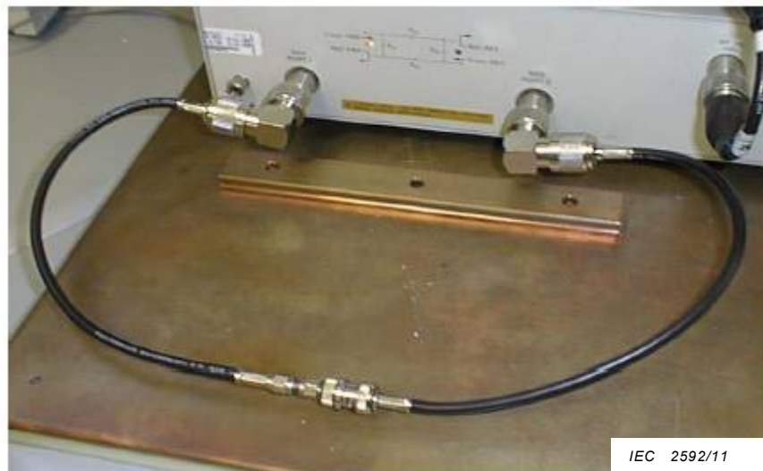
Figure 10 – Coaxial lead attenuation calibration
