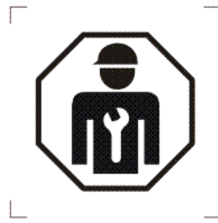
IEC 60417-6183:2013-09 Installation, mechanical expertise
