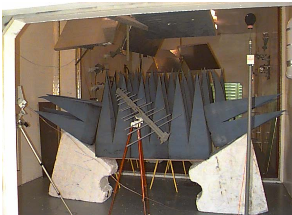
Figure A.14 – Distribution of absorbers for loading effects test
