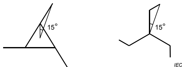
Figure 4 – 15° phase shifting is preferably realized by extended delta or zigzag connection
