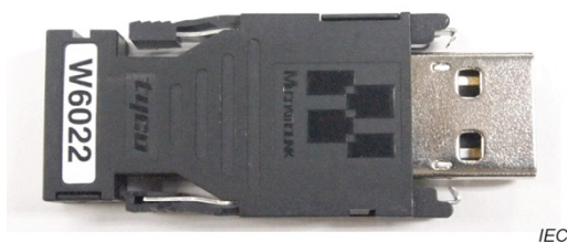
Figure A.10 – Terminator installed in M-II cable connector
