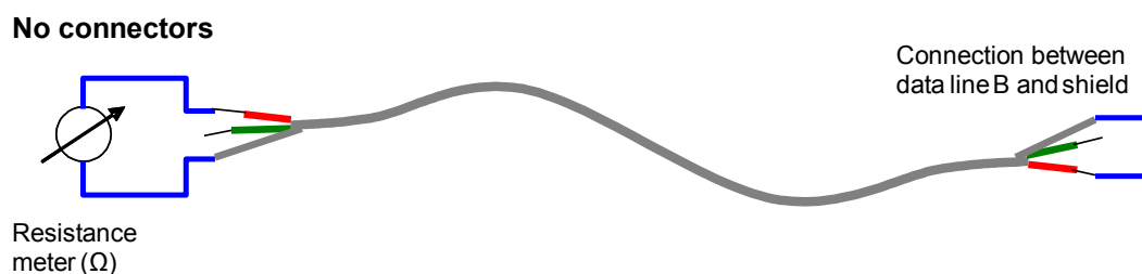
Figure A.9 – Resistance measurement without 9-pin Sub-D plug
