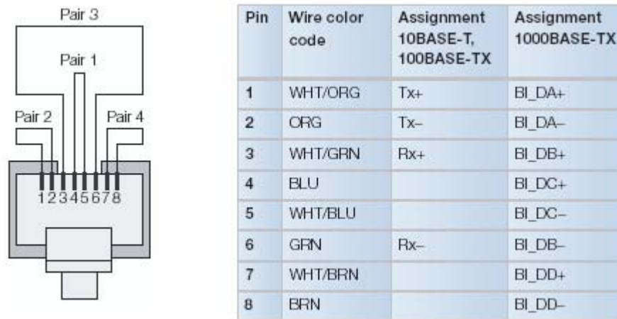
Figure 13 – RJ45 pin assignment
