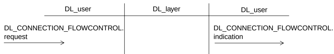
Figure 17—Timing sequence diagram for DL layer flow control primitives
