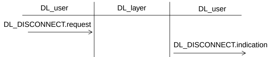
Figure 18—Timing sequence diagram DL layer disconnection primitives
