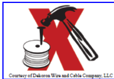
Figure 4-00 not nail into reel flanges
