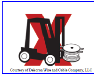
Figure 6-00 not lift reels by the top flange
