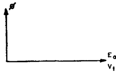
Figure I-1 Alternating-Current Generator Field Flux and Armature Voltage Vectors—No Load.
