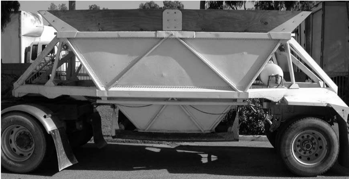
Figure 4—Example of a bottom dump
