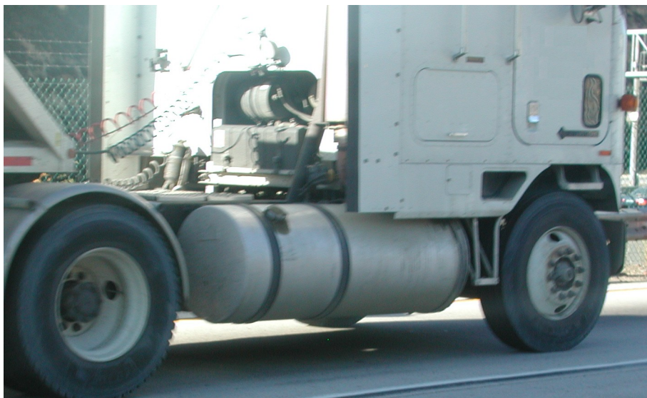
Figure 17—Example of a saddle tank
