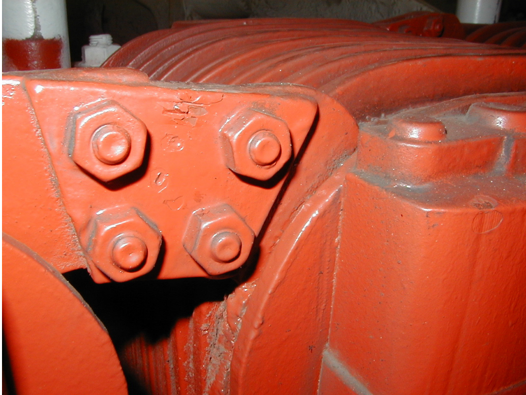
Figure 5—Straight solid copper tabs
