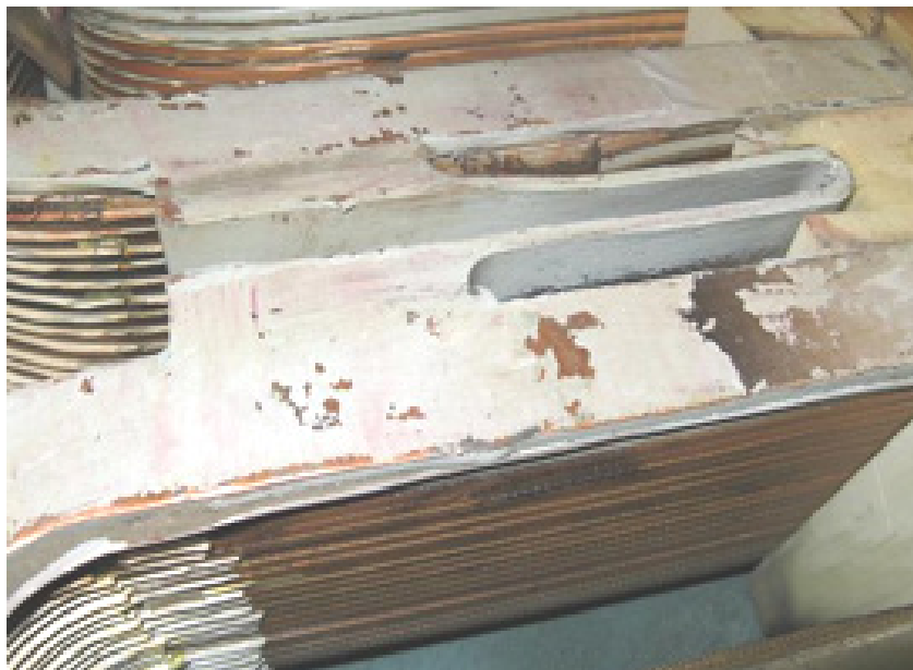
Figure 3—Omega-type solid copper connector
