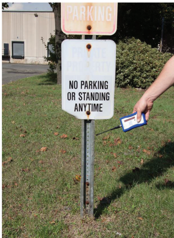
Figure 19—The use of a hand-held electric field detector to locate energized objects
