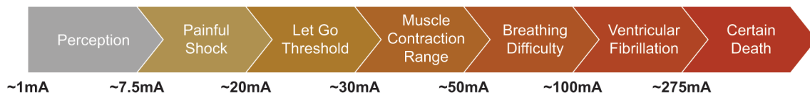
Figure 1—Effects of 50/60 Hz electric current on body (3s contact)
