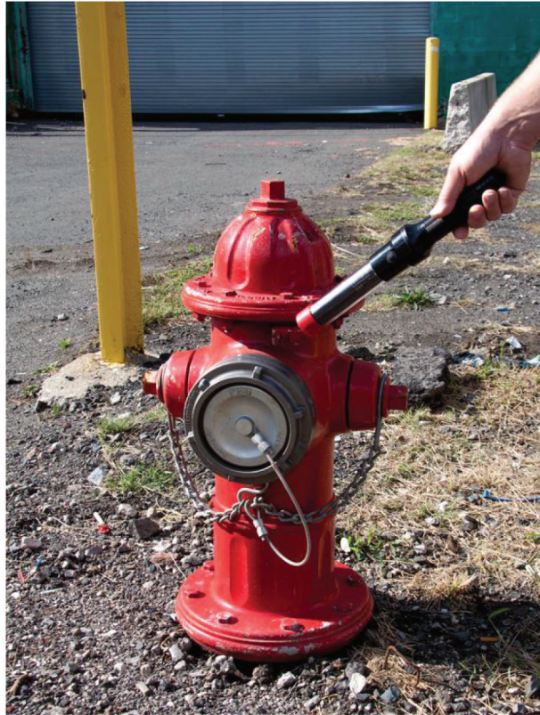
Figure 18—Using a hand-held electric field detector to check for the presence of electricity on a candidate reference
