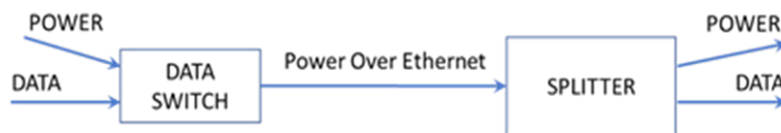
Figure 1—Basic schematic diagram of PoE
