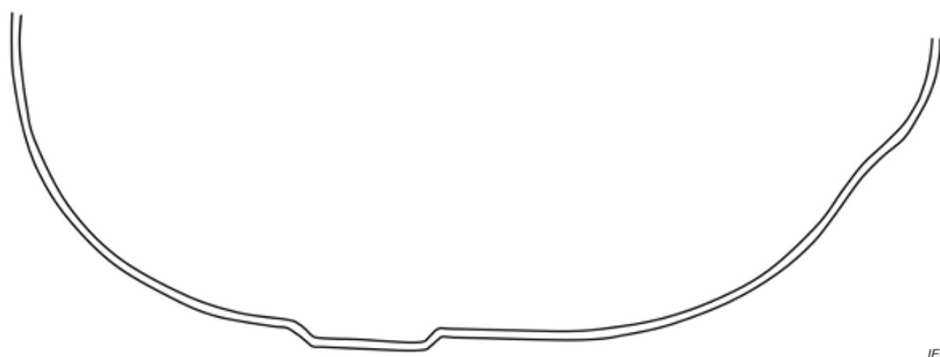
Figure 4 – Cross-sectional view of SAM virtual phantom for PD evaluations at the reference plane (shell thickness is 2 mm everywhere, including at the pinna)
