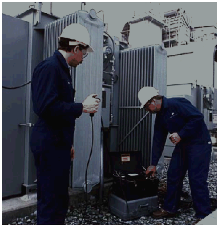
Figure 6-2—Insulation power-factor testing
