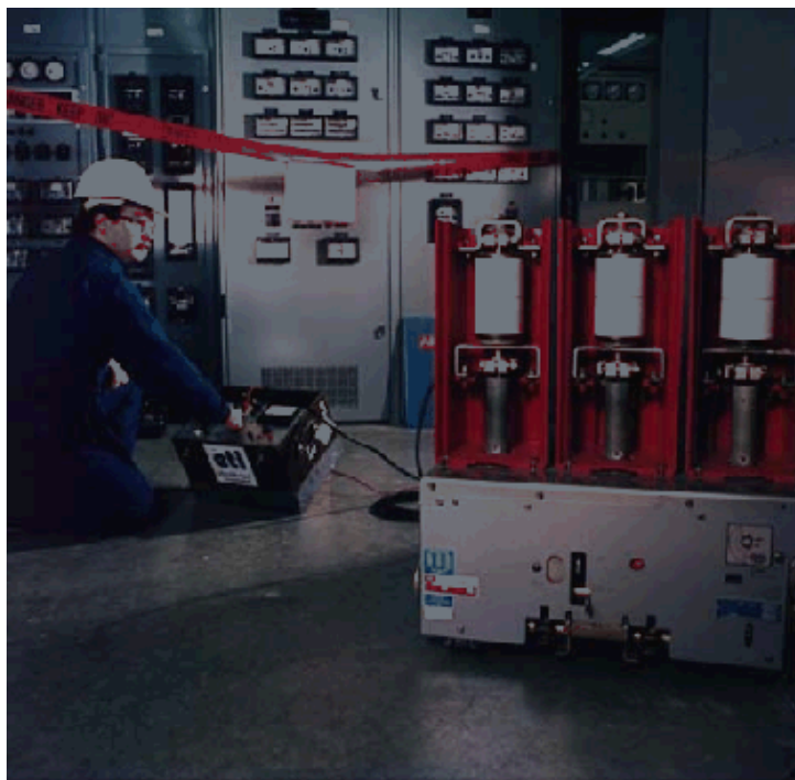
Figure 6-1 — Circuit breaker high-potential testing
