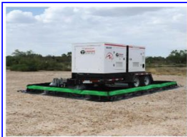
Figure 6—Containment for a mobile generator
