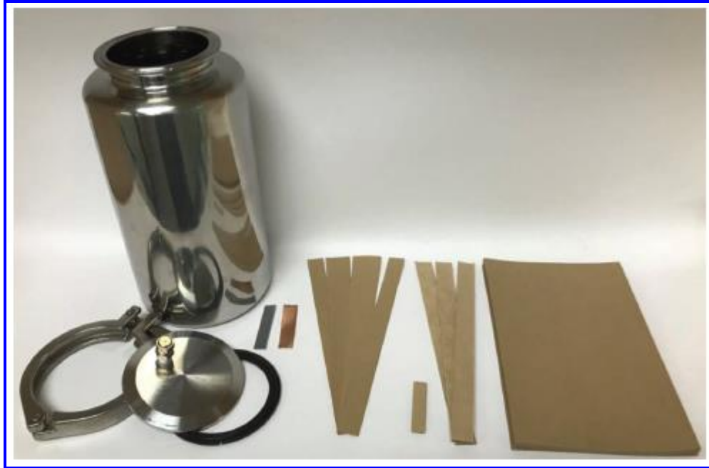
Figure 3—“2 liter” stainless steel container with associated hardware, including lid with installed pressure relief valve, lid clamp, and single-use high-temperature sealing gasket compatible with the insulating liquid
