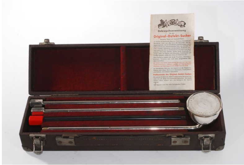
Figure 5—“Original Defekt Sucher,” mechanical Instrument to investigate structural sound (~1930)
