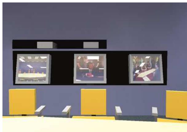
Figure 3. Veiling reflections on VDT displays
