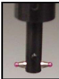
Internal thread measuring ball stylus
