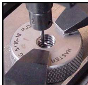
Ball stylus engaged on one side of ring
