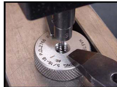
Ball stylus engaged on opposite side of ring
