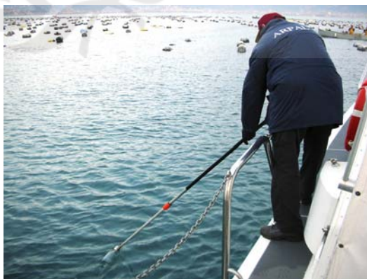
Figure 2 – Sampling superficial water for oil detection close to mariculture activity
