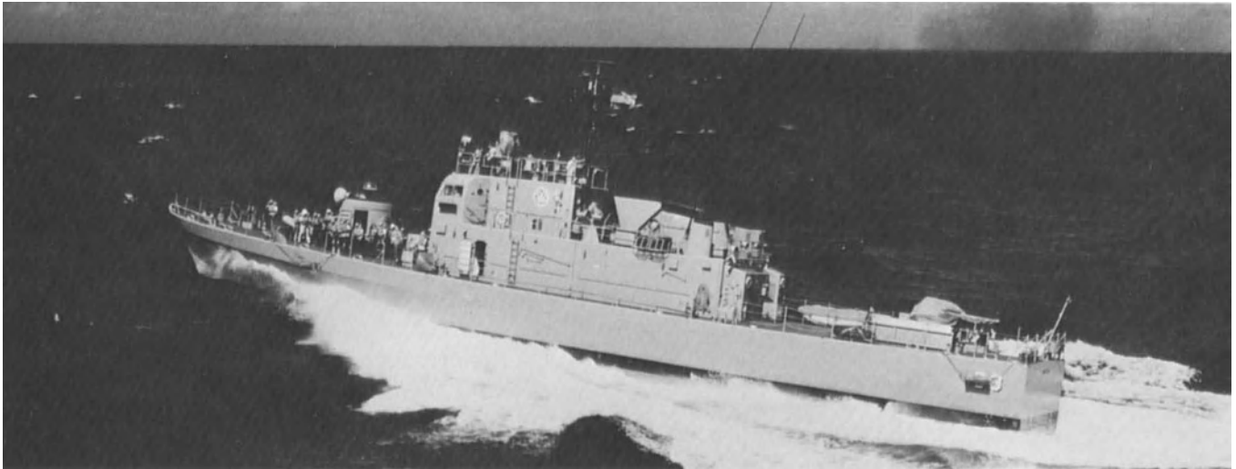
Figure 1-5. The USS Welsh , a fast navy gunboat, is capable of planing speeds but has a combination power plant more economical for cruising at lower speeds. She thus operates as a semiplaning hull.
