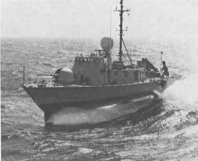
Figure Figure 1-3. The hydrofoil-supported vessel. These craft have the best seakeeping potential of the various hydrodynamically supported vessels.
