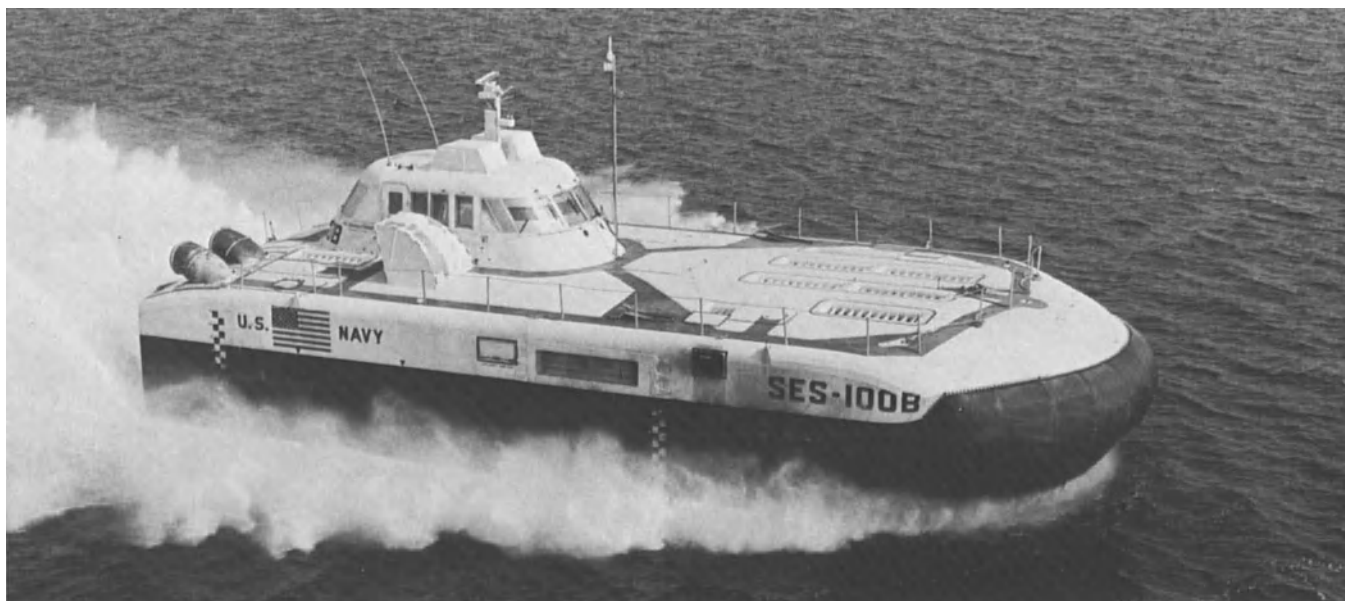
Figure 1-1. A one-hundred-ton surface effect ship, an air-cushion vehicle (ACV), making a test run. These vessels are supported on a cushion of relatively low-pressure air supplied by ducted internal fans. They are propelled at potential speeds up to 80 knots by turbine-driven water jets. (Courtesy of Bell Aero Space Co.)
