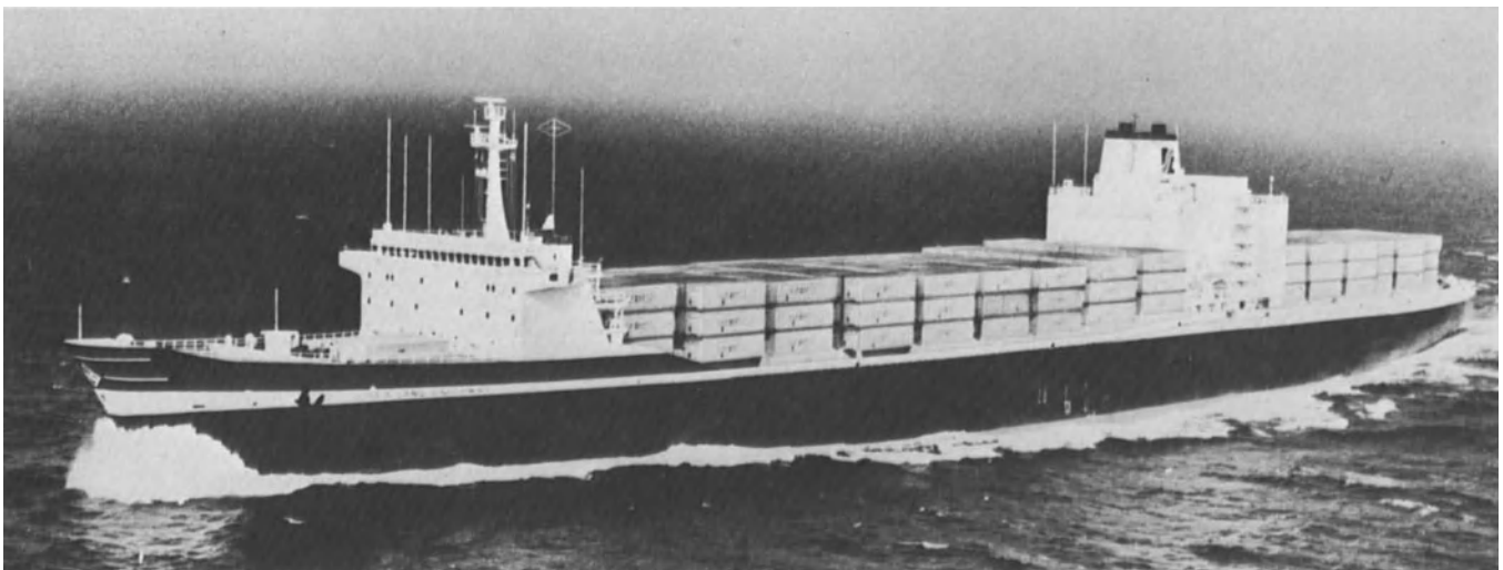
Figure 1-7. The hard-working and valuable displacement ship of the SL 7 type is currently the fastest cargo ship in the world, capable of sustained cruising speeds of 33 knots. (Courtesy of Sea-Land Industries, Inc.)
