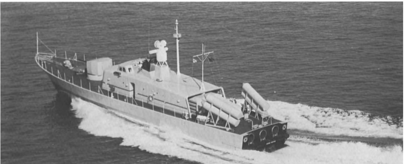
Figure 1-4. HMS Tenacity , a fast fisheries patrol vessel, is essentially a planing hull. A large example of this type, she is 142 feet long, powered by gas turbines, and capable of 40-kt speeds. She was originally intended as a fast surface-to-surface missile carrier. (Courtesy of Vosper-Thornycroft, Ltd.)
