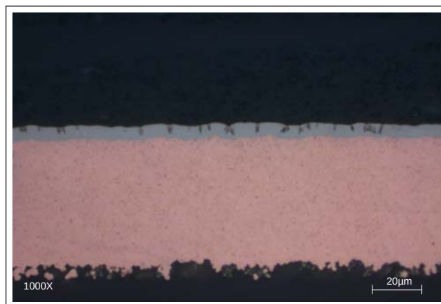
Figure 3-32 Level 3 Hyperactive Corrosion – SMT Feature at 1000X
