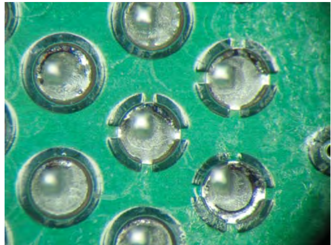
Figure 3-13 Another Example of the SAD Defect
