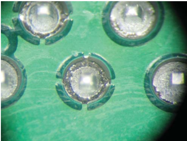
Figure 3-12 Example of SAD (Selective Annular Ring Dewetting)
