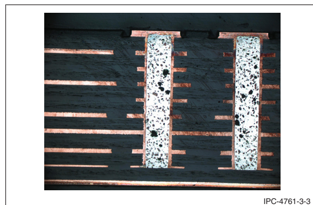
Figure 3-3 Voids in Via Fill Material
