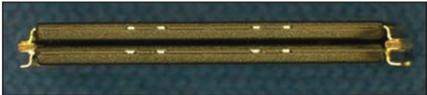
Figure 4-13 Stacked Thin Small Outline Package (TSOP) Devices
