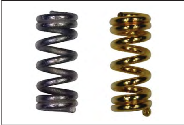
Figure 4-18 SnPb-Plated Microcoil (Left) and Au-Plated Microcoil (Right)
