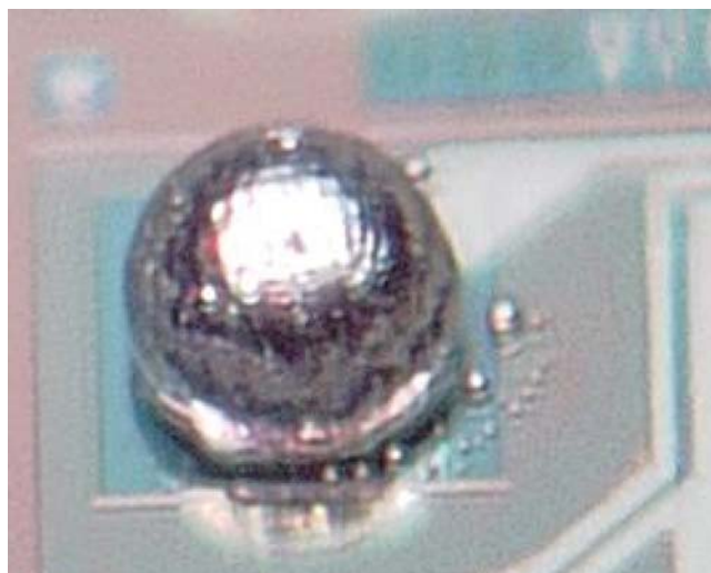
Figure 1-5 Solder Balls Following Solder Reflow
