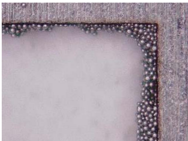
Figure 1-3 Solder Paste Buildup on Walls of Stencil Apertures
