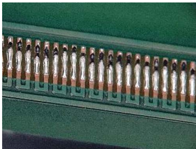
Figure 1-4 Open or Insufficient Solder Joints
