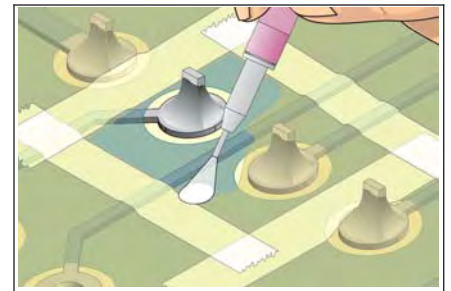
Figure 2 Remove coating using micro blasting system.
