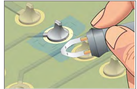
Figure 1 Apply thermal tip to soften or granulate the material.
