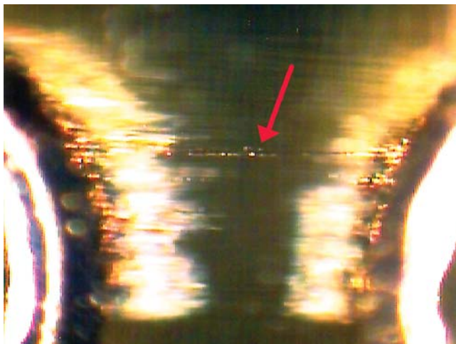
Figure 4-3 Failure Analysis Photo Showing Suspected CAF Failure Between Very Closely-Spaced Plated Through Holes c
