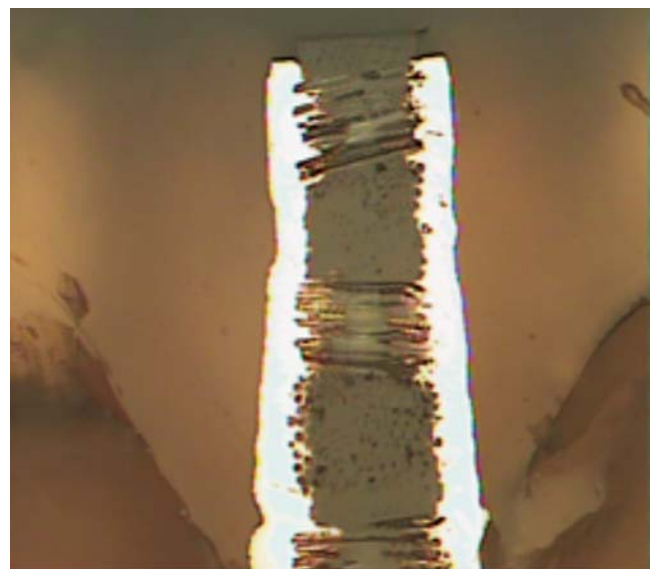
Figure 8-2b Damage Due to Hole Drilling and Wicking
