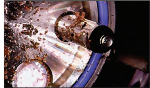
Figure 5-1 Contamination (Oil and Debris) Figure source: Fiber Optic Precision Cleaning
