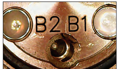
Figure 5-3 Contamination (After Cleaning) Image Credit: Fiber Optic Precision Cleaning
