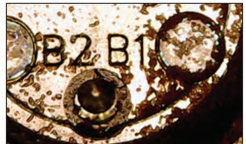
Figure 5-2 Contamination (Before Cleaning) Image Credit: Fiber Optic Precision Cleaning
