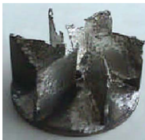
Figure 3-10 Lead-free Solder Alloy Attack of Wave Solder Equipment ("Pb-free Technology and the Necessary Changes in Soldering Process and Machine Technology," H. Schlessmann, APEX 2002 Conference Proceedings)
