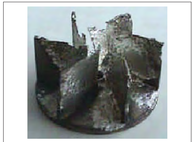
Figure 3-10 Pb-Free Solder Alloy Attack of Wave Solder Equipment ("Pb-free Technology and the Necessary Changes in Soldering Process and Machine Technology," H. Schlessmann, APEX 2002 Conference Proceedings)
