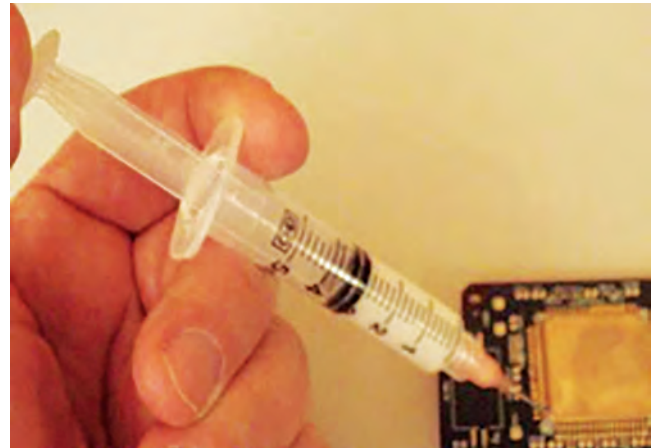
Figure 3-4 Dispensing Via Manual Syringe
