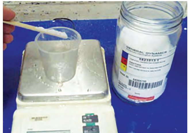
Figure 3-1 Example of a Silica Filler Being Added to Epoxy as a Percentage by Weight
