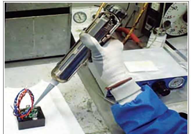
Figure 3-5 Dispensing Via Air-Assisted Caulking Gun
