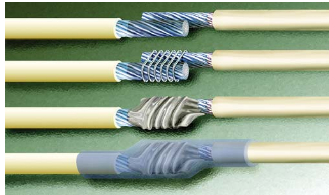
Figure 5-10 In-Line Lash Solder Splice Image Courtesy of NASA
