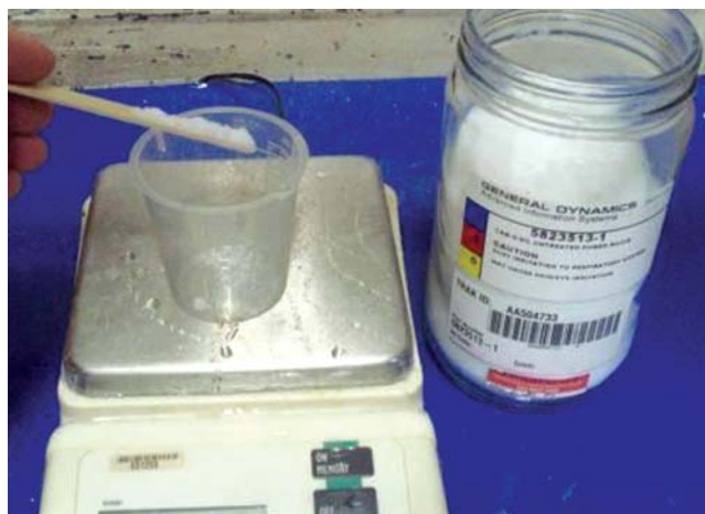
Figure 1-5 Example of a Silica Filler being added to Epoxy as a Percentage by Weight
