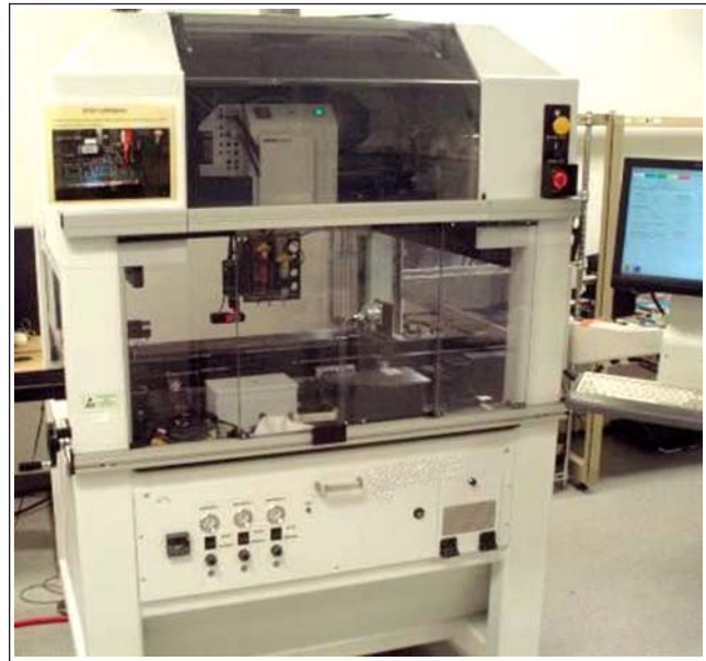
Figure 1-20 Dispensing via Fully Automatic X-Y-Z Axis Computer Controlled Systems (Image Courtesy of GPD Global)
