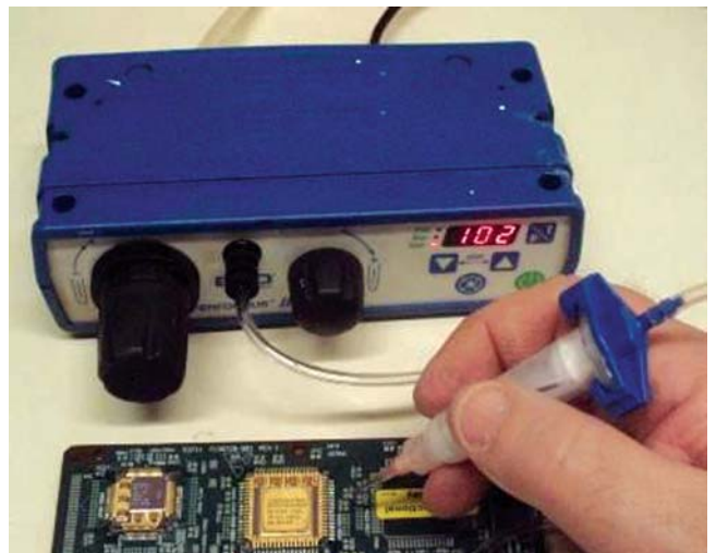
Figure 1-19 Dispensing Via Time/Pressure Controlled Manual Dispenser (Image Courtesy of Nordson EFD)
