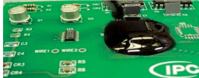
Figure 1-2 Injecting Potting Material onto a Module (Encapsulation)
