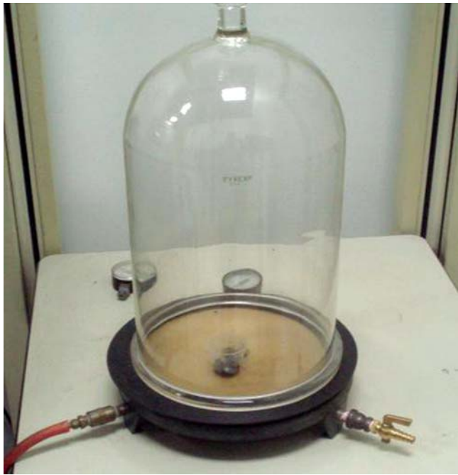
Figure 1-15 Bell Jar Vacuum Pump (Used for evacuating air bubbles from mixed epoxies prior to or after encapsulation)
