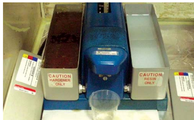
Figure 1-27 Metered Mixer. This system will dispense a two-part epoxy mixed to the desired (set) ratio. Shown with the reservoir covers removed for clarity.
