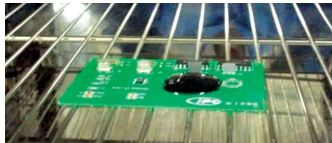
Figure 1-3 Encapsulation Curing in Oven
