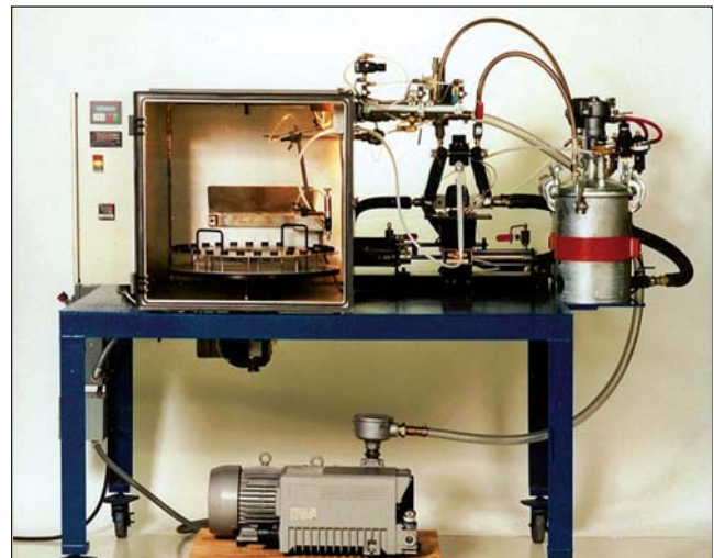
Figure 1-14 Unit which is capable of degassing an assembly
