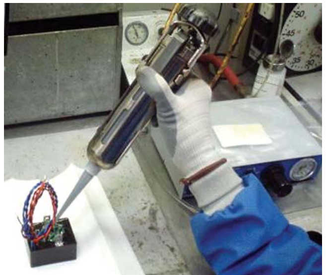
Figure 1-18 Dispensing Via Air Assisted Caulking Gun
