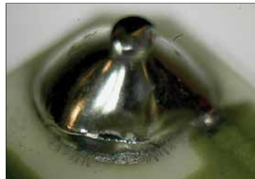
Figure 3-4 A SAC 305 solder joint with Silver dendrites [Figure courtesy of Spur Electron and Ultra Electronics, UK].
