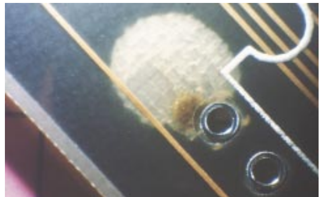
B-24 Blistering adjacent to land Delamination
