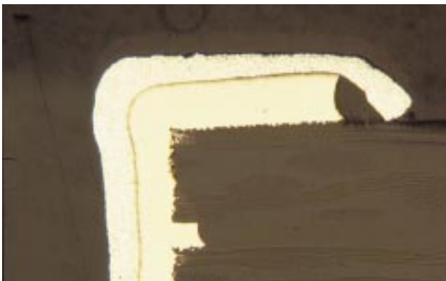
C-9 Conductor undercutting collapse
