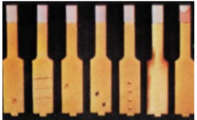
D-4 Gold contacts Pit, pin holes and surface nodules
