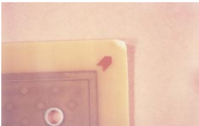
A-3 Corner damage
