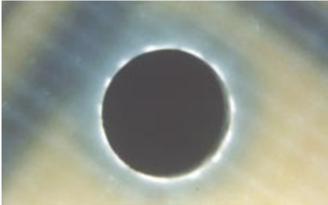
B-1 Unsupported hole Haloing
