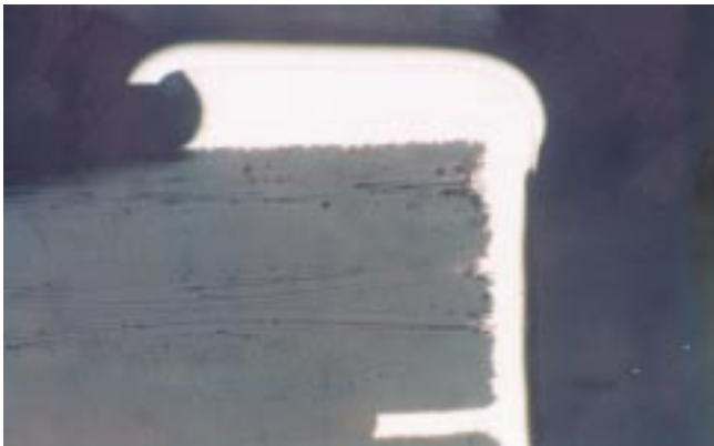
C-8 Conductor overhang
