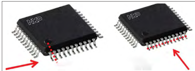
Figure 6 Metallographic Cross-Section Angles: Profile (left), End (right)
