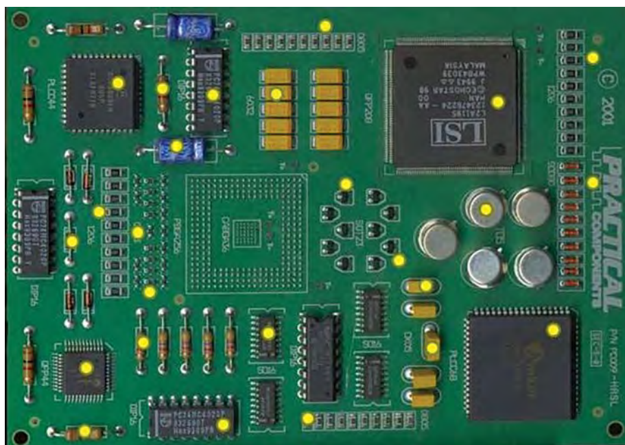
Figure 7 PC009 Board with Components Selected for Metallographic Analysis
