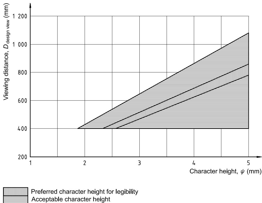
Figure 11 — Viewing distance — character size relationship
