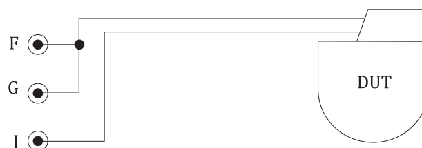
Figure 6 — Differential mode connection to single-channel bipolar device
