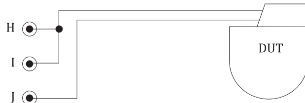
Figure 17 — Differential mode connection to a single-channel bipolar device
