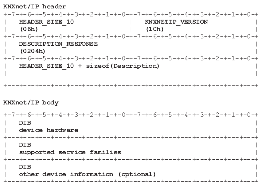
Figure 29 — DESCRIPTION_RESPONSE frame binary format
