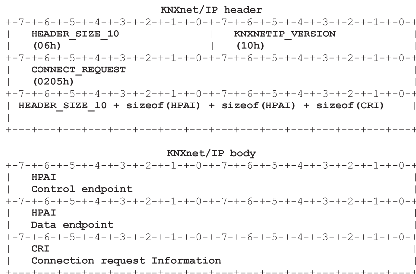
Figure 30 — CONNECT_REQUEST frame binary format
