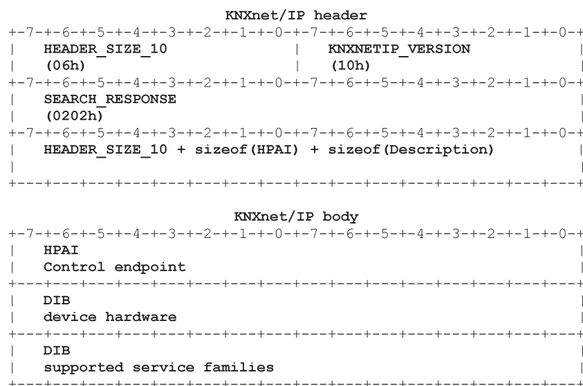
Figure 20 — SEARCH_RESPONSE frame binary format
