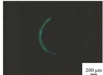
Figure 5 — Examples of C-crack with chordal angle < 180^\circ
