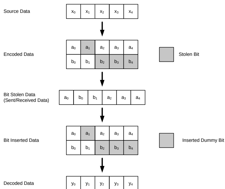
Figure 20 - An example of bit-stealing and bit-insertion for R=5/6 code
