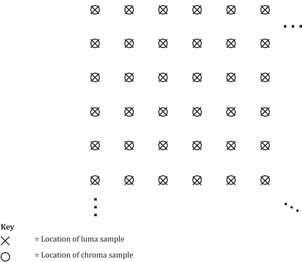
Figure 3 — Nominal vertical and horizontal locations of 4:4:4 luma and chroma samples in a picture
