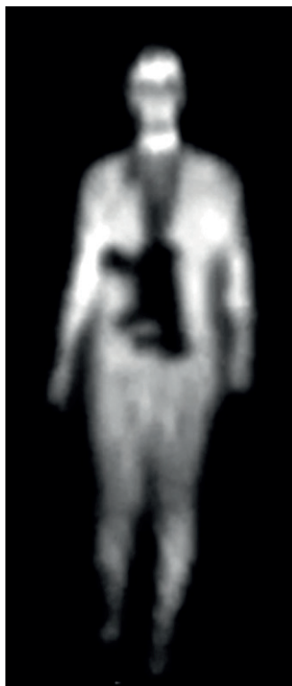
Figure 11 — Submillimetre image showing a gun hidden under subject's clothing
